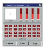
The test screen is fairly self-explanatory. Across the top are displays for up to 6 axes, below that is a display for up to 32 buttons. The actual number of axes and buttons which are displayed depends on the device that's currently being tested, so you will probably see less than what is shown in the above graphic.
